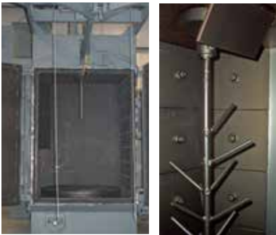
Examples of manganese wear plates (X120Mn12) for shot blasting cabinets.
